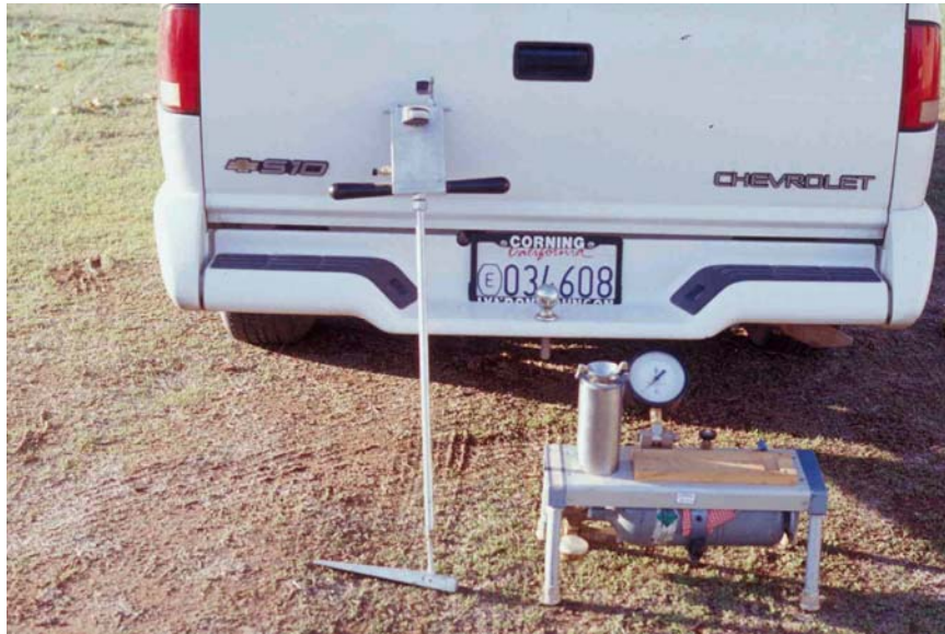
Figure 1. Example of manually operated "pump-up" pressure bomb (left) and pressure bomb console (right).
