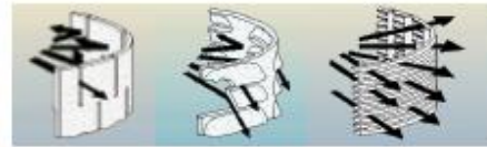
Figure 2. Mill slot, louver, and wire wrap screen (left to right).
